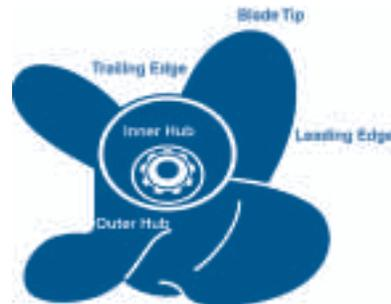
Common outboard engine propeller
