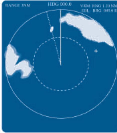
This drawing shows how a vessel can be pointing in a direction away from you, yet still presents a risk of collision. The radar will help you determine this.
