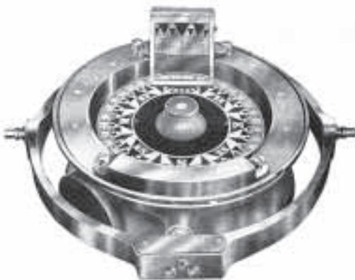
The compass is an essential tool of navigation. It is not a complex device, but it can confuse an operator, sending a vessel off in the wrong direction. The compass card always points towards magnetic north, thus
