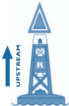
Starboard Hand Buoy
