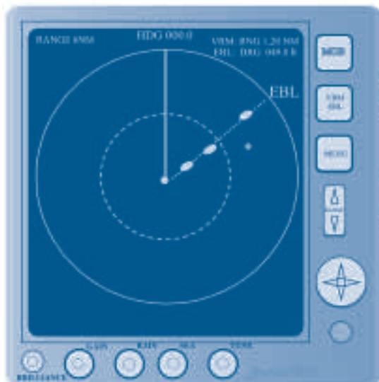
The target has a steady bearing and a decreasing range. The Electronic Bearing Line or EBL is used to track the target's advance.
