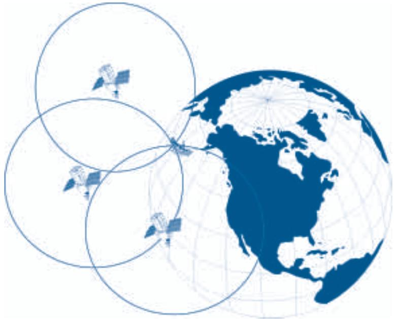
rived from onboard atomic clocks) on two frequencies, L1 and L2. A separate channel on each frequency is dedicated to each satellite.
