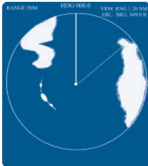
Side Lobe Error. This is caused by the beams side lobes reflecting off the target at short range.
