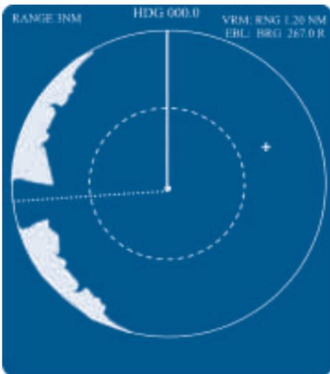
Low valleys or wet lands can appear as channels or inlets. A common mistake is for navigators to be expecting to see an opening and turn when the radar screen looks like this (this is actually a beach with a valley behind it).
