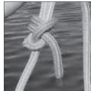
Inspect your lines before use. (Note the frayed strands)
